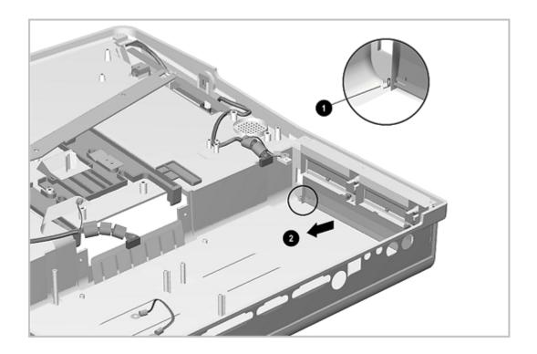
Figure 7-25. Removing the MultiBay Door
